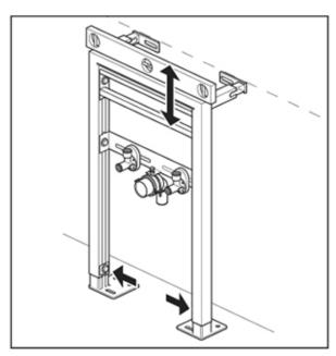
Place the frame against the wall in the required position.
