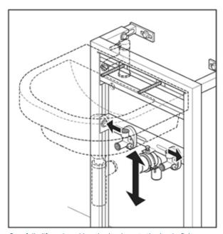
Carefully lift and position the basin onto the basin fixing bolts. Loosen the connection height adjustment bolts, set the connection support bar to the required height to line up with the waste outlet elbow. Retighten the bolts and remove the basin.
