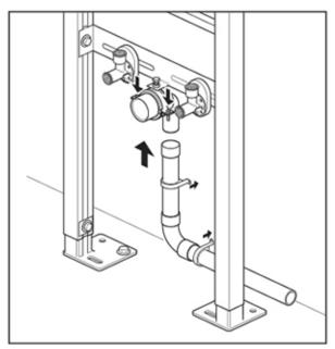
Prepare and connect the waste water outlet (a push-fit waste is recommended).
