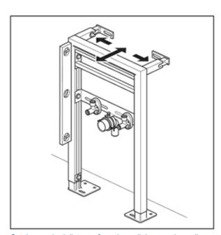
Set the required distance from the wall. Loosen the wall adjustment bolts, set to the required distance, check the frame is vertical and retighten the bolts.
