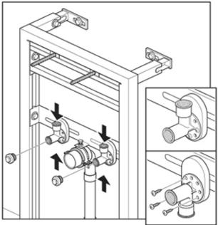
Connect the hot and cold pipework to the inlet elbows (Ø ½"), screw the blanking plugs into the outlets. BSP female threaded outlets may need extending using male nipples. The hot and cold inlet elbows can be rotated as required to suit your pipework. It is essential that isolaton valves are fitted at this point.
