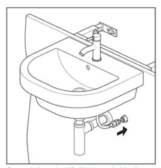
Connect the hot and cold flexible pipes to the inlet elbows, adaptors may be required.
