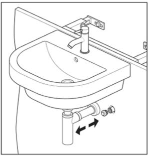
Secure the outlet pipe onto the trap and slide the cover up to the wall.
