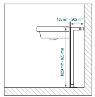
Plan the position of the basin. The recommended basin height is 850 mm to the front rim.
