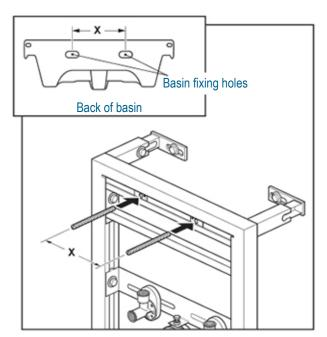
Measure the distance 'X' between the centres of the basin fixing holes. Insert the basin fixing bolts into the sliding plates, position centrally on the frame and space apart to match the basin fixing holes. Tighten the fixing bolts with a large screwdriver and cut to length if required.
