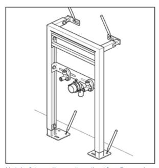
Mark the fixing positions on the wall and floor. Remove the frame and drill suitable holes for the fixings.
