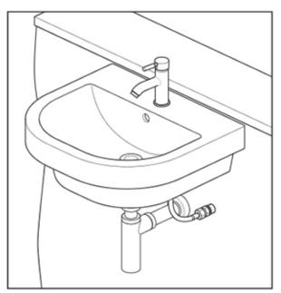
Finish the installation by water testing the inlet and outlet connections in the void.
