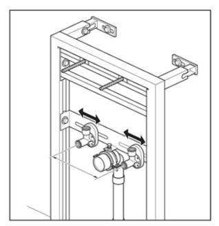
Loosen the hot and cold inlet elbows (using the nut at the rear), set to the required distance apart and retighten.
