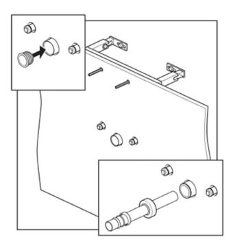
Push fit the waste pipe seal into the waste outlet elbow. Build the partition wall, making the holes for the bolts and pipes as small as possible. If required, tile the surface or apply the finish now. Lubricate the inside of the waste pipe seal and push fit the basin waste pipe fit into the waste outlet elbow.
