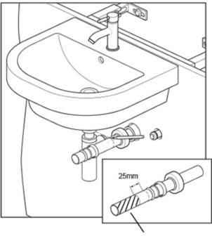
Carefully position the basin on the wall, mark a line level with the end of the waste trap outlet onto the basin waste pipe. Remove basin and waste pipe, add a further 25 mm to the length of the waste pipe and cut to length. Some extension pipes are stepped at the trap end, ensure the correct end is cut and any burrs are removed. Refit waste pipe into waste outlet elbow. The above applies to the 'Bathstore cylindrical trap'.
