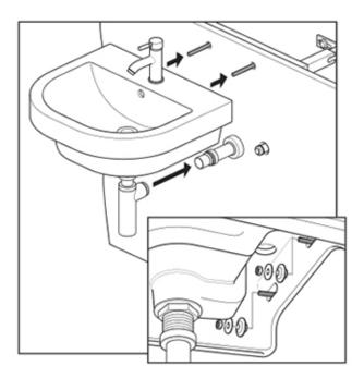
Carefully position the basin onto the fixing bolts, lining up the waste connections at the same time.
